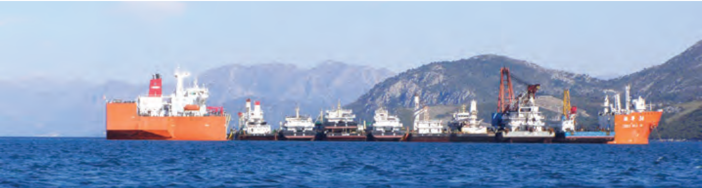
March 2019: vessels for bridge construction were delivered to the construction site by a semi-submersible naval vessel.
