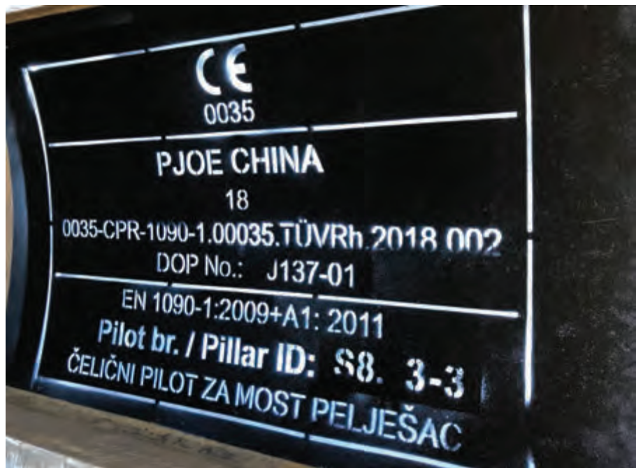
The production of piles in the Chinese factory was certified according to the EU regulation, therefore the manufacturer was able to put the CE construction product mark on them
