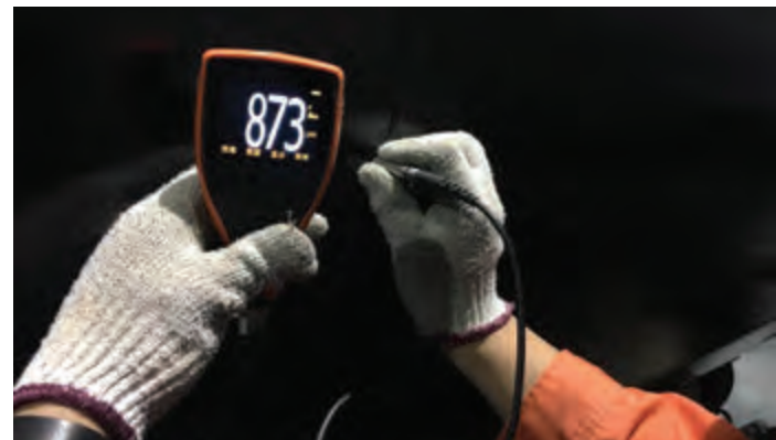
Testing the thickness of anti-corrosion protection of the piles of the Pelješac Bridge, the default thickness is 850 µm
