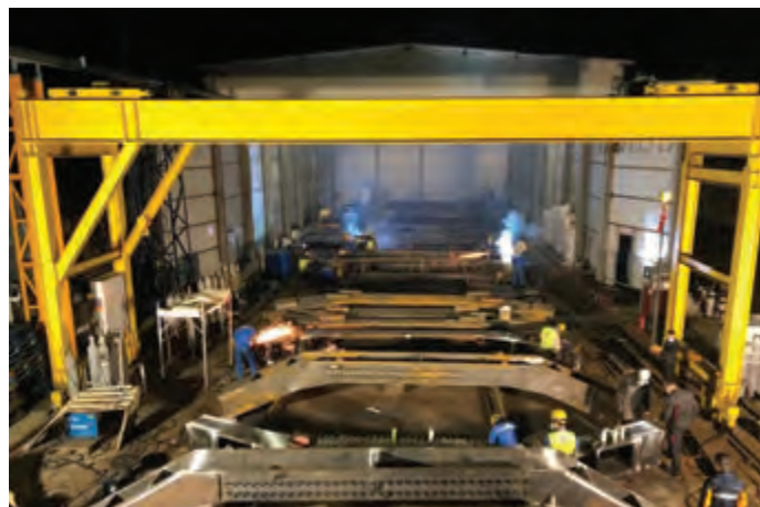
Production of pylon saddles in the factory
