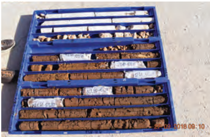
Samples from the seabed at the location of the future bridge foundation are placed in a box in order, that is, according to the depth from which they were taken. The boundary between the poorly bearing clay and the rock is visible at a depth of 127 m, or about 100 m below the seabed.
